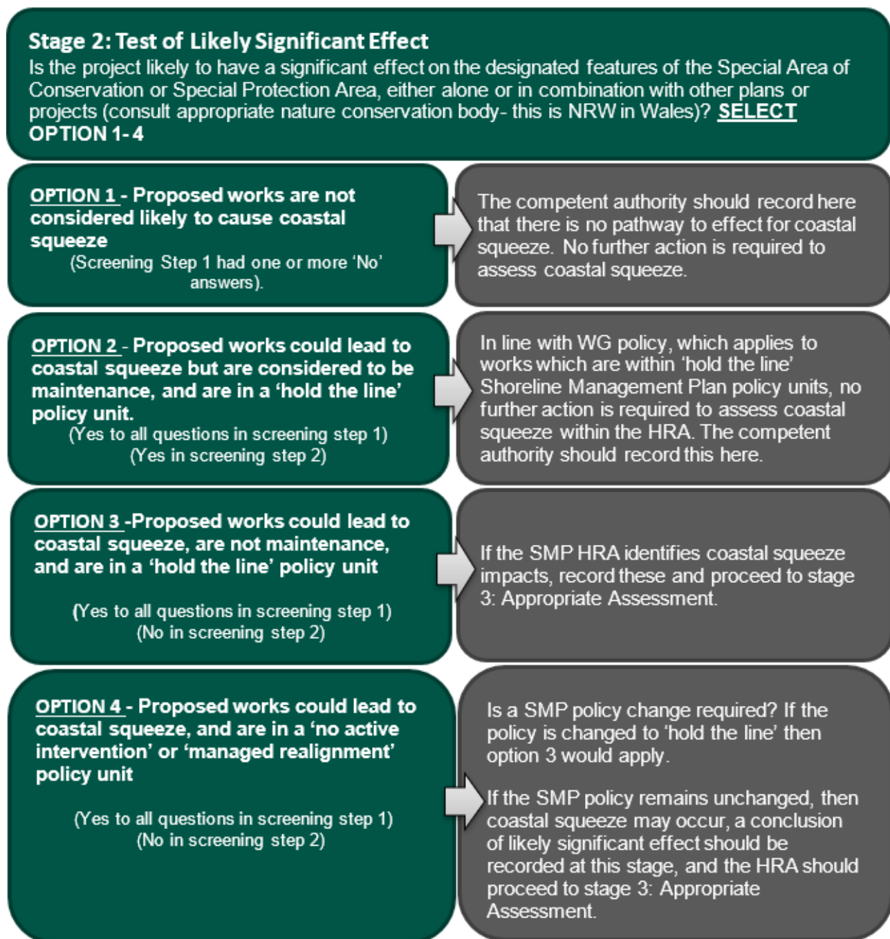
Figure 4 Flow chart to explain the options under Stage 2 (Test of Likely Significant Effect) of the HRA
