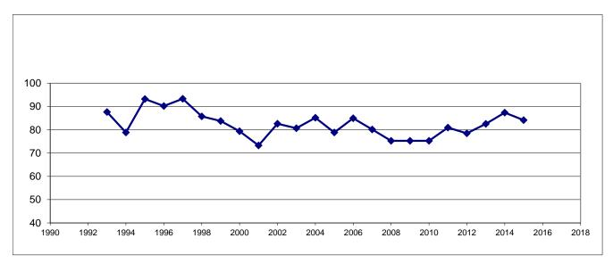
The maximum gust recorded for 2008, 2009 & 2010 was exactly the same (75.28 knots). It is possible the bearings were faulty. The bearings were replaced in 2011 and higher gusts are now being recorded. 2015 saw a maximum gust of 84.17 knots.
