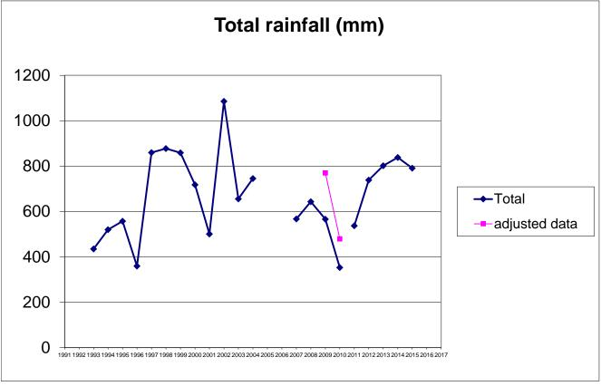
There was some extreme weather in February 2014 with 100mph winds recorded on the 12<sup>th</sup> Feb 2014. The rain gauge recorded 199mm of rain for that day. – It is most likely that this was a false reading. The winds will have vibrated the rain gauge causing it to "tip" when there was no water in the bucket.
