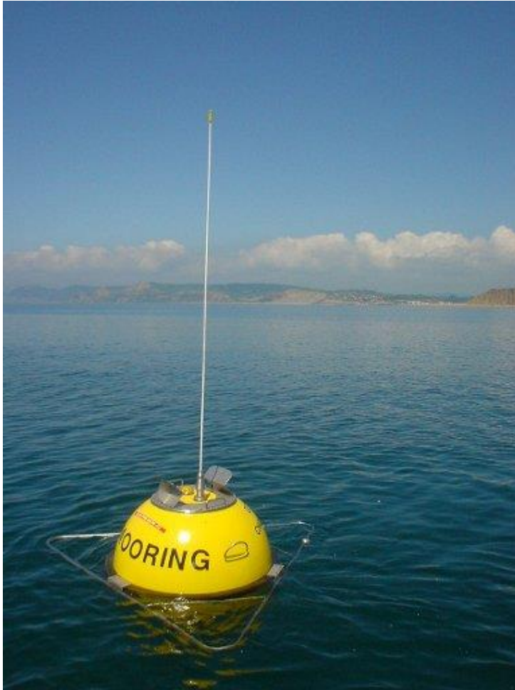
Figure 18: Directional waverider buoy in West Bay (Regional Coastal Monitoring Programme).
