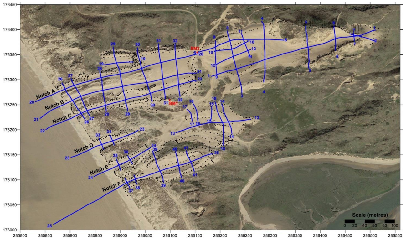
Figure 2. Locations of March 2015 data points (black dots), benchmarks (red dots) and cross-profiles (blue lines), overlaid on air photographs flown 18 April 2015 (source: Google Earth).
